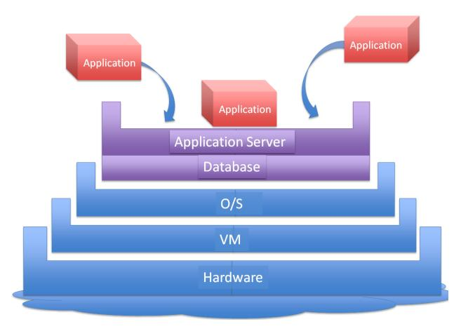
The infrastructure that a cloud can provide consists of hardware on which typically virtual machines will run that contain an operating system to run applications as well as storage devices for persisting data.
